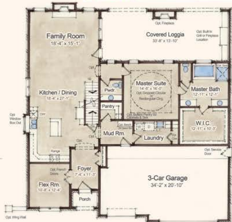
First Floor Plan 1,914 sq. ft. 9" Standard First Floor Ceilings. Interior Radius Archways Are Optional.
